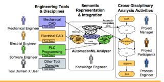
The AutomationML Analyzer enables efficient integration, browsing, querying, and cross-disciplinary analysis of diverse engineering models represented as *AutomationML* data.
